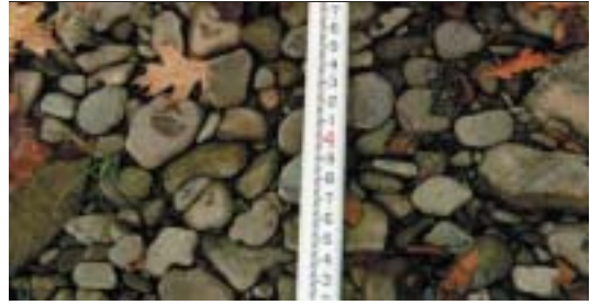
The bed of Bear Creek contains cobble and boulder sized particles derived from siliciclastic bedrock formations in the Appalachian Plateau Province.
