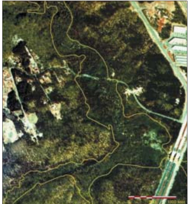
The floodplain limits of Severn Run. Note the reduced width of the floodplain as it passes under the I-97 highway (lower right). These types of constrictions can cause water to back up on the upstream side and increase flow velocities immediately downstream during flood events.
