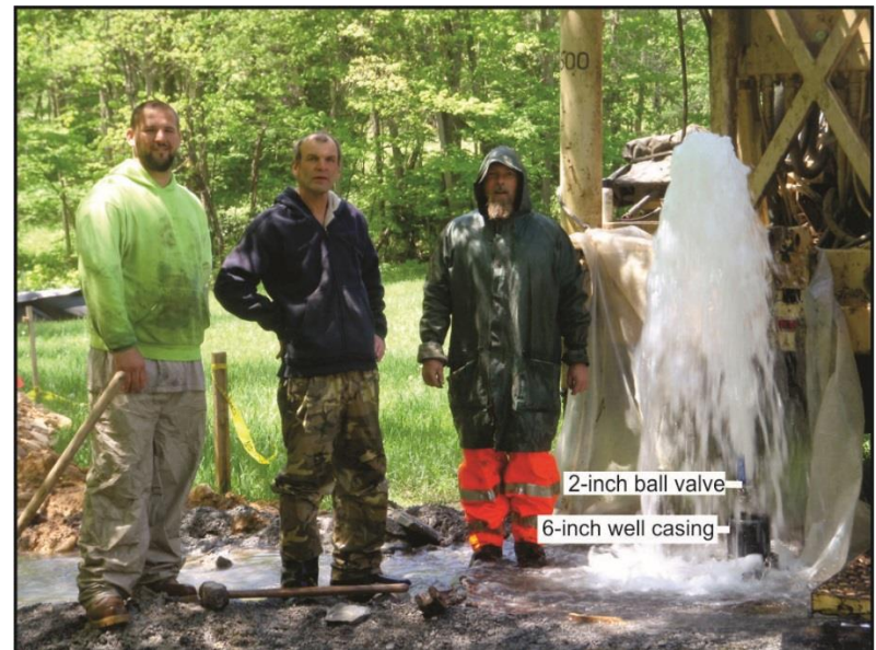
Figure 6. Flowing-well conditions for well GA Aa 15 (Deep well) at the Buffalo Run test site (May 19, 2014).
