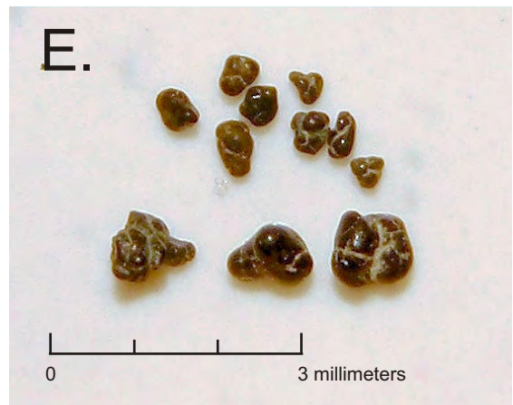
Figure 3. Photomicrographs of Aquia aquifer sediments: A. Washed sand. B. Quartz grains: iron-stained (left), clear (right). C. Calcite: cement (left), shell fragments (right). D. Goethite grains. E. Glauconite grains. Sample from well CA Db 96, 580 to 600 feet.
