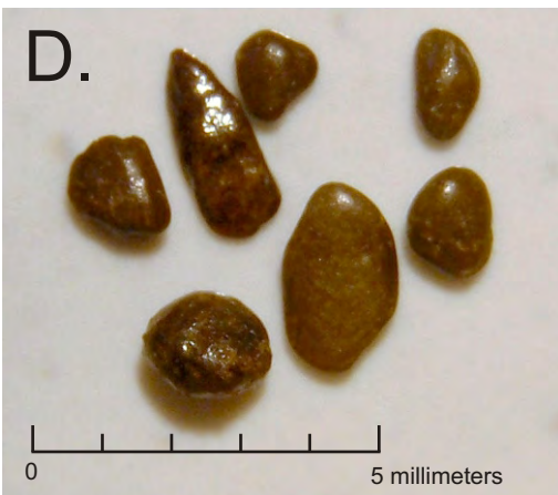
Figure 3. Photomicrographs of Aquia aquifer sediments: A. Washed sand. B. Quartz grains: iron-stained (left), clear (right). C. Calcite: cement (left), shell fragments (right). D. Goethite grains. E. Glauconite grains. Sample from well CA Db 96, 580 to 600 feet.
